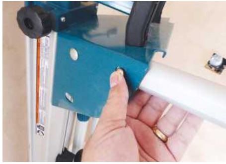
▲ Depressing this button allows the legs to be opened or closed
